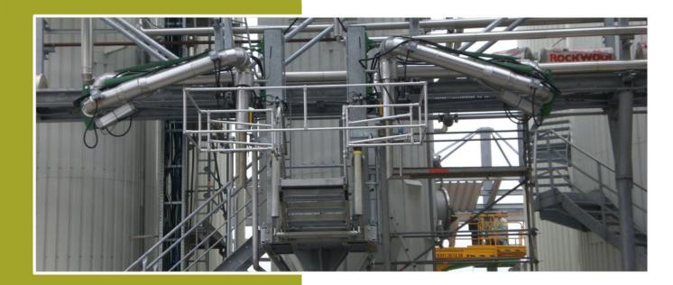
**IGATEC Top Loading Systems** are used for the safe and fast loading and unloading of railcars, road tankers, sedimentation tanks, trailers and any other suitable tanks from above.
